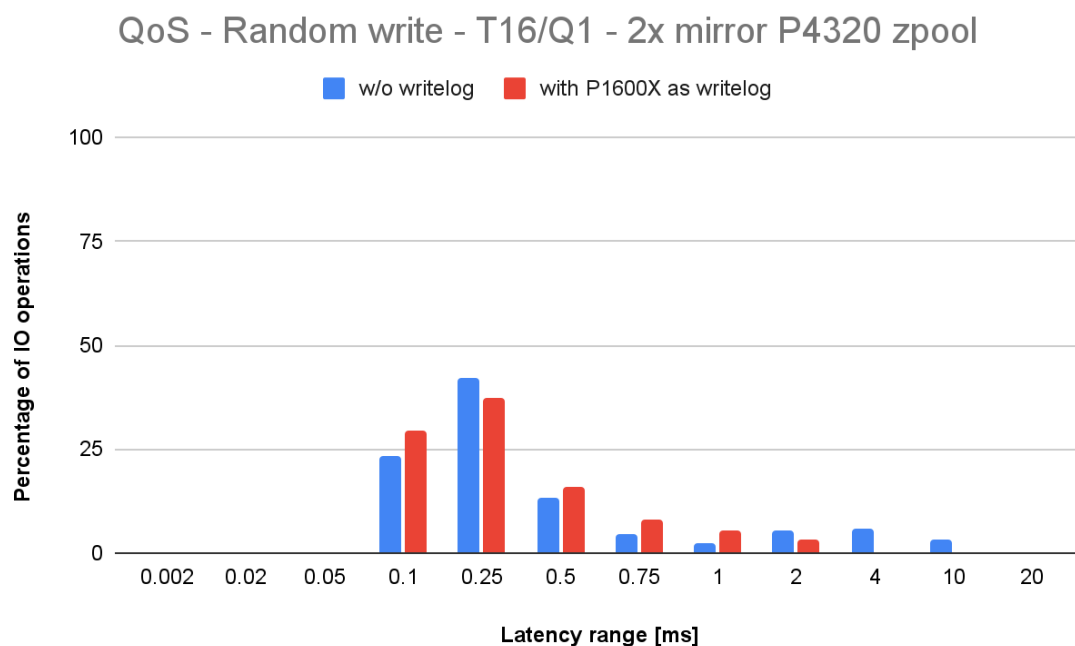
Fig. 24. Latency distribution for a random write test, done on a 2x 2-way mirror SSD zpool (T16/Q1), with and without writelog.
