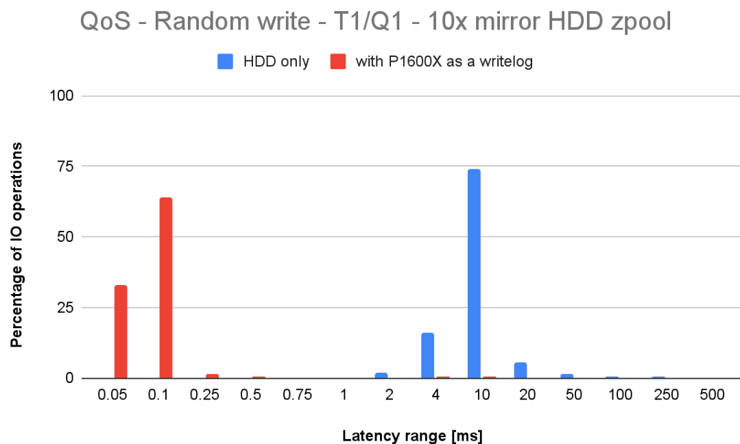
Fig. 11. Latency distribution for a random write test, done on a 10x mirror HDD zpool (T1/Q1), with and without writelog.
