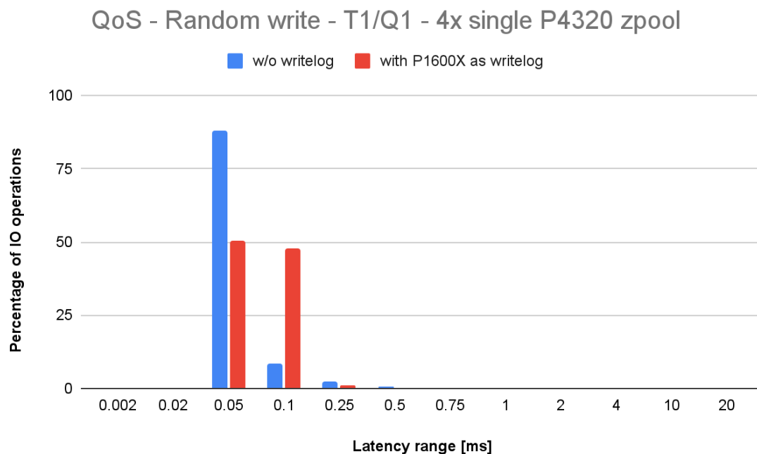
Fig. 29. Latency distribution for a random write test, done on a 4x single SSD zpool (T1/Q1), with and without writelog.
