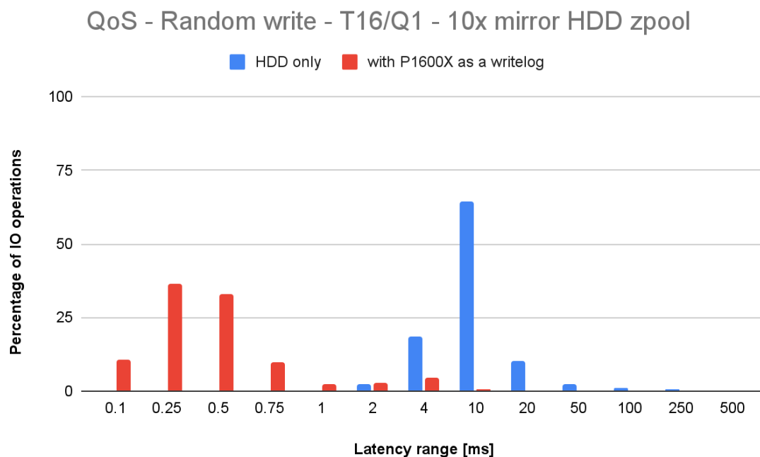
Fig. 12. Latency distribution for a random write test, done on a 10x mirror HDD zpool (T16/Q1), with and without writelog.
